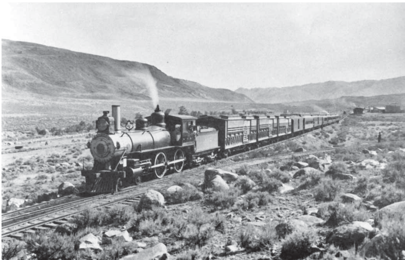
Some time during September of 1896, Frank Jay Haynes took a photo of a train leaving Cinnabar, heading north to Livingston. The engine is a Webb Special and the first cars were designed to carry horses. MONTANA HISTORICAL SOCIETY RESEARCH CENTER
